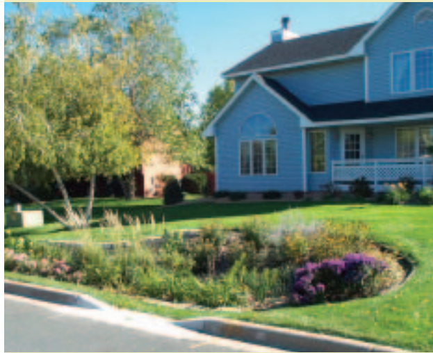
Rain gardens are beautiful and they can help save our rivers and lakes. This rain garden in the City of Burnsville reduces stormwater volume by 92%! PHOTO COURTESY OF BARR ENGINEERING.
